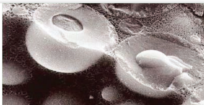
Microcapsules frozen at -70°C showing the frozen protective colloid ( 40.000 X electronic microscope )
