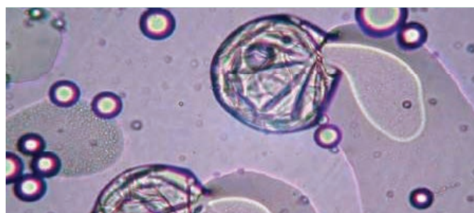
Micro capsules releasing active ingredient by disruption or diffusion (1.000x enlarged) big capsules produced specially to show the release of the A.I. No example of the actual commercial product.
